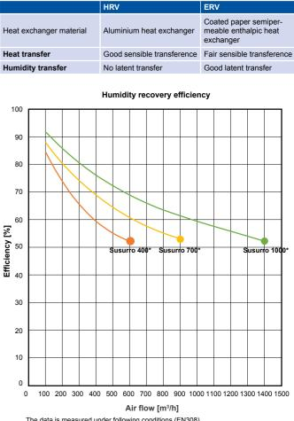
The data is measured under following conditions (EN308) Outdoor air temperature is +5°C, relative humidity 72% Indoor air temperature is +25°C, relative humidity 28%
